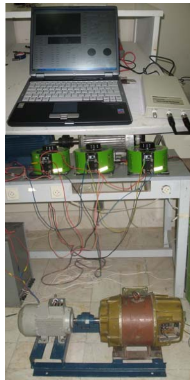
Fig. 4. Experimental Test setup: Motor-Generator System (Right) and data acquisition system (left) [8]
