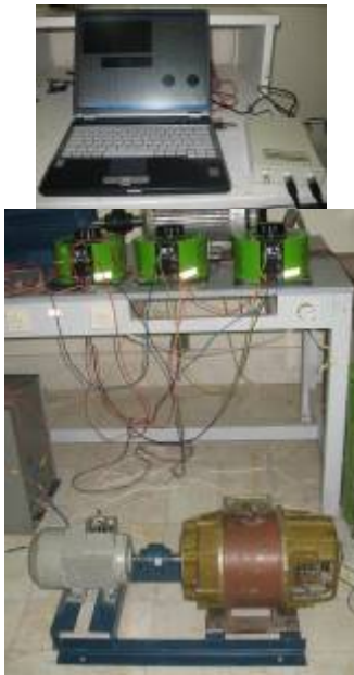
Fig.4 Experimental Test setup: Motor-Generator System (Right) and data acquisition system (left) [5]
